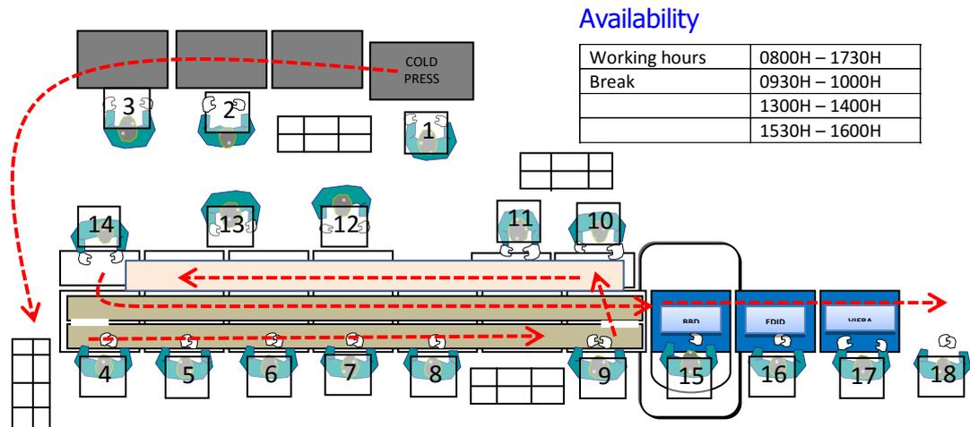
Figure 1: The flow of the current production line
