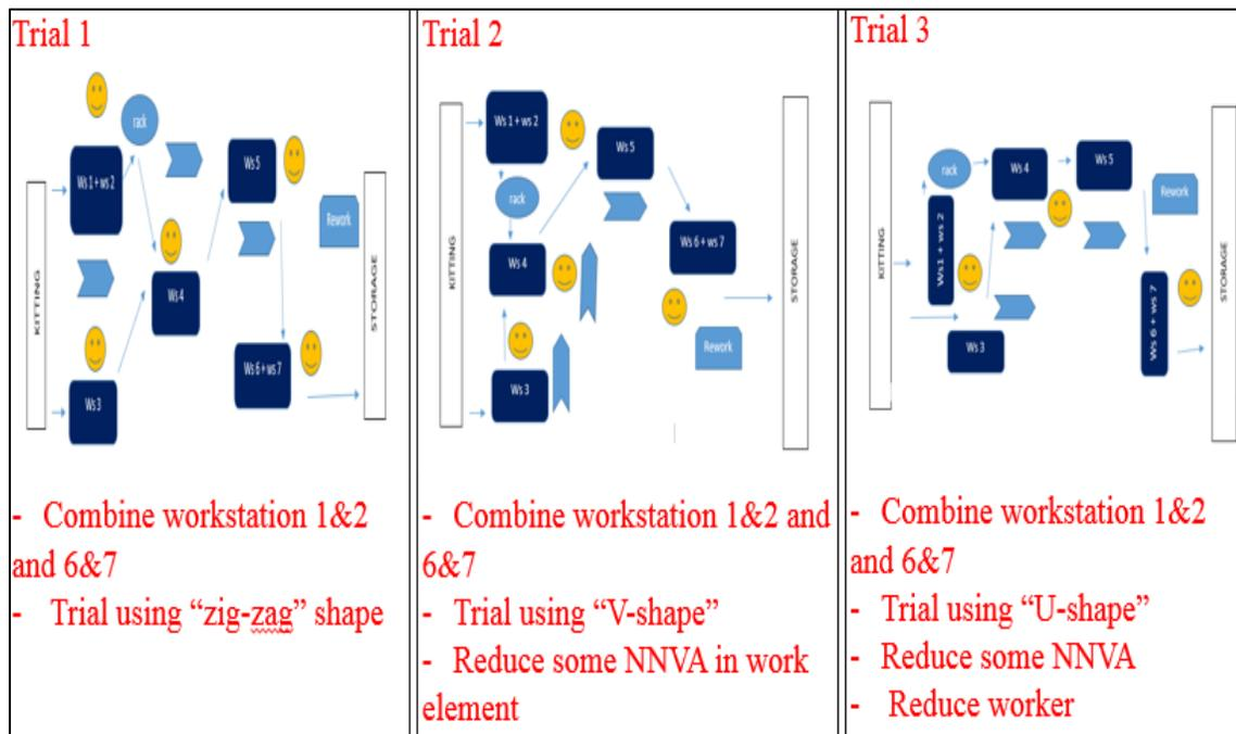
Figure 3: Trial’s using Cellular Layout
