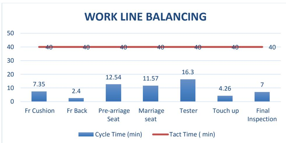
Figure 2: Actual Layout Line Balancing
